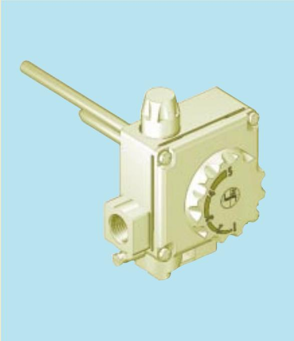
**Multifunctional safety control with thermoelectric flame failure device, pressure adjuster with override device and on-off thermostat. No external electric power supply required.**
